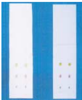
Left : Chromato Sheet Right : Silicagel 70F 254 Plate-wako Sample : Wakogel B-Tester (#231-00051) Developing solvent : Chloroform
