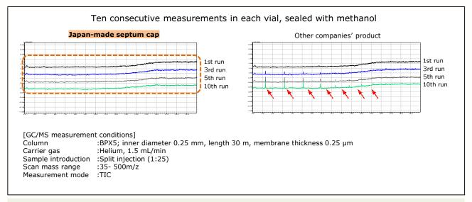
In consecutive measurements, leachables observed with other companies' products were hardly detected with Japan-made septum cap. Leachables from a cap or septum can have unexpected effects on test results, such as appearance of ghost peaks. Thus, it is necessary in analytical testing to pay attention to the quality not only of vials, but also of septum caps.
