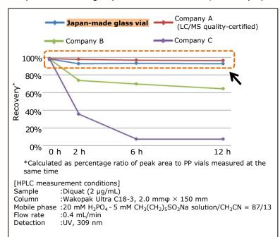
Diquat adsorption to Japanmade glass vial was hardly observed up to 12 hours, demonstrating as low adsorption as LC/MS certified high-quality glass vials from other companies. As sample adsorption to vials causes sample loss, use of lowadsorption vials is important to avoid problems in analysis.
