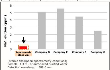
Japan-made glass vial was shown to be associated with low Na<sup>+</sup> elution. As elution of alkaline components from vials causes sample decomposition, etc., it is critical to pay attention not only to sample adsorption to vials, but also elution from vials.
