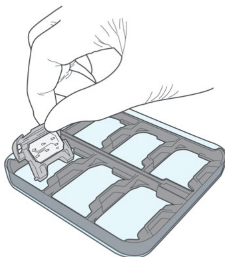
Figure 1. Place chips by sliding under the tab of the Chip Cradle
