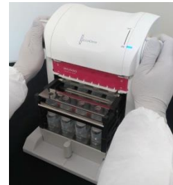
Turn Rotary Switch to pressurize the first row
